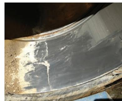
*Under the same process conditions, the competitor's valve underperformed and required frequent maintenance due to erosion.*
